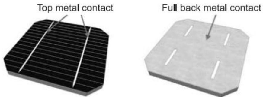
**Figure 3.1.** Front side and back side of a silicon solar cell
