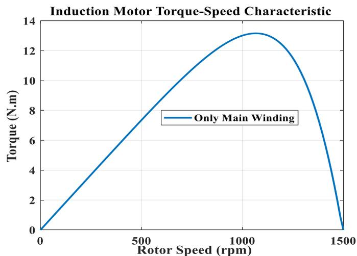
**Figure 3.12.** Torque-speed characteristic only main winding SPIM
