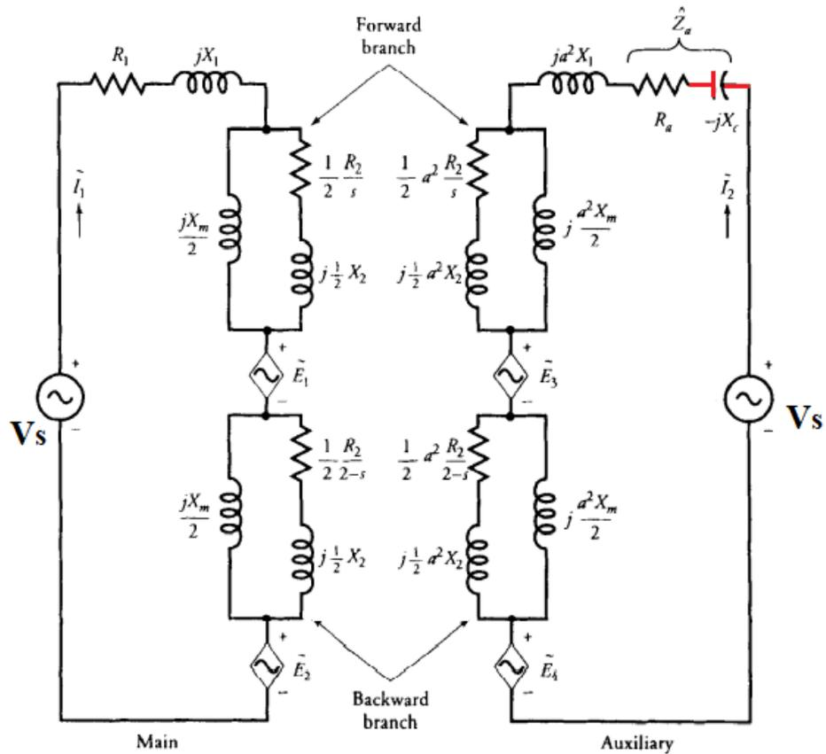
Figure 3.13. Equivalent circuit of the main winding and auxiliary windings of a capacitor-start induction motor
