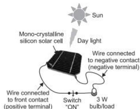
**Figure 3.2.** Solar cell with terminals and load
