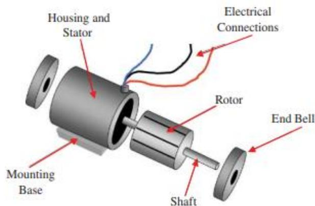
**Figure 3.7.** Construction of the single-phase induction motor.
