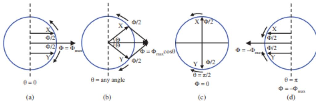
**Figure 3.9.** The flux that was produced in relation to the angle
