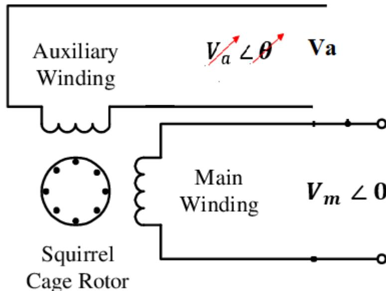
**Figure 4.1.** Schematic diagram of single-phase induction motor powered by two different voltage sources
