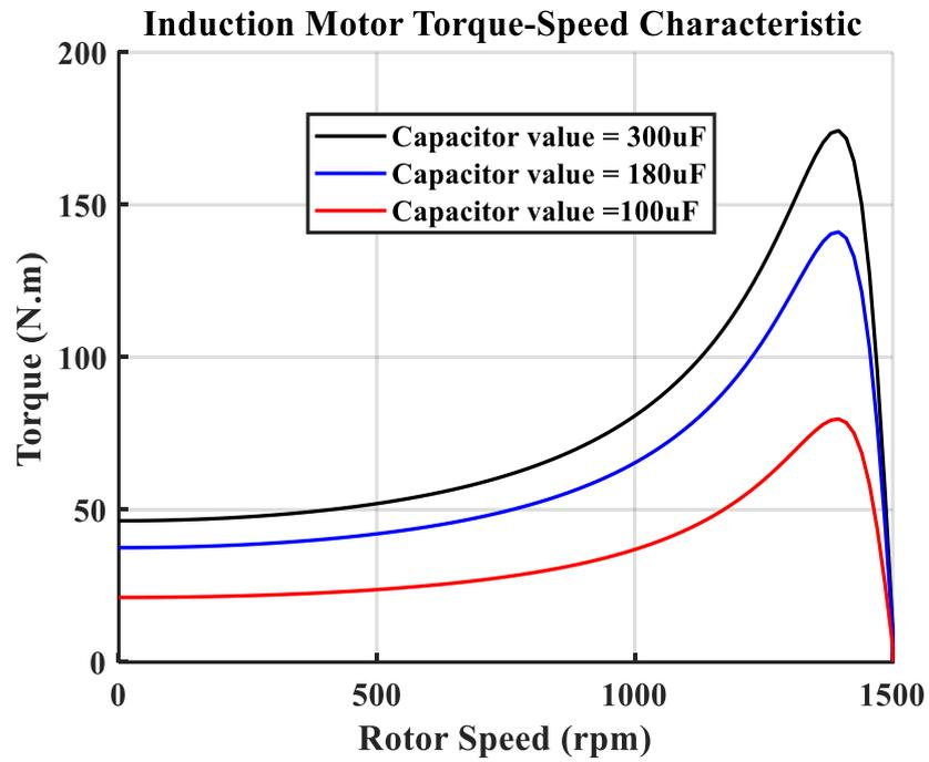
**Figure 3.14.** A Capacitor-start induction motor's torque-speed characteristic
