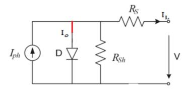
Figure 3.3. Photovoltaic equivalent circuit
