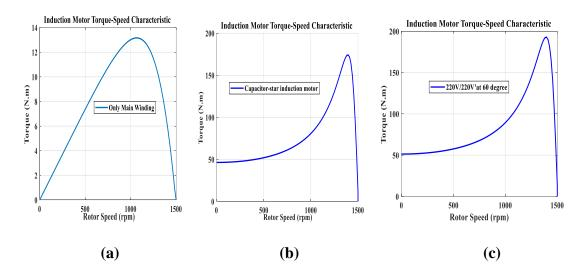
**Figure 5.1.** Torque speed characteristics of SPIM; **a**) SPIM with only main winding; **b**) Capacitor-star SPIM; **c**) SPIM with two voltage sources
