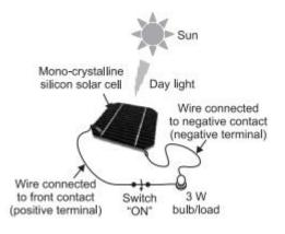
Figure 3.2. Solar cell with terminals and load
