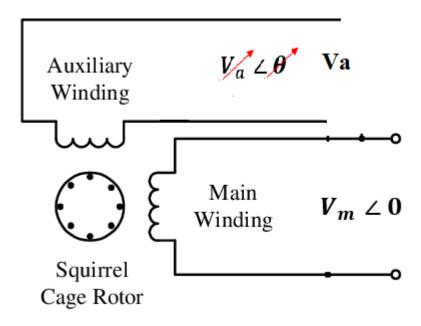
**Figure 4.1.** Schematic diagram of single-phase induction motor powered by two different voltage sources
