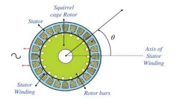
Figure 3.8. Cross-sectional view of a single-phase induction motor
