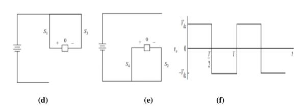
Figure 3.5. a) Full-bridge inverter; b) S1 and S2 closed; c) S3 and S4 closed; d) S1 and S3 closed; e) S2 and S4 closed; f) Output voltage of full bridge inverter
