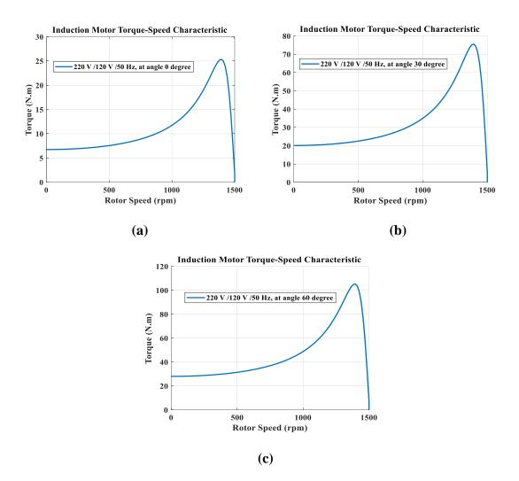
Figure 4.4. Phase angle between the two windings of the motor; a) At angle 0-degrees;b) At angle 30-degrees; c) At angle 60-degrees
