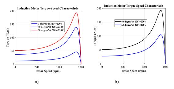
**Figure 5.2.** Torque speed characteristics of SPIM **a**) By controlling the phase angle; b) By controlling the voltage supply for the auxiliary winding
